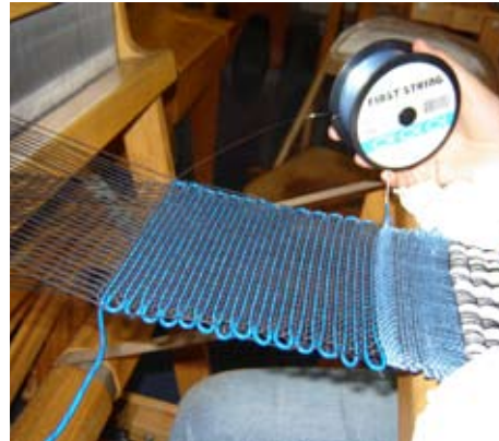
I wove fishing line in between the electro-luminescent wire in order to make it look like there was more ambient light without using more of the glowing wire. This dropped its price point.
