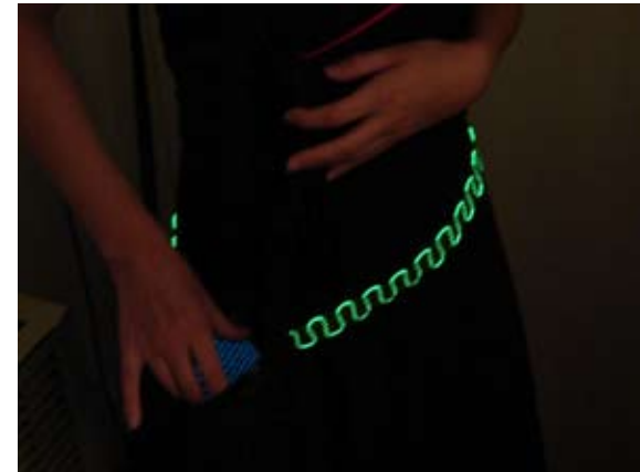
Elweave would work great as a pocket insert for purses or bags. It would make finding your keys easy at night. Because of its low frequency, the light has a strobe effect when moving.
